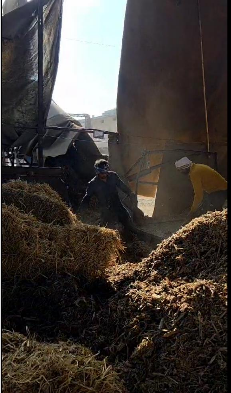
Bagasse being fed into Conveyor Belt
