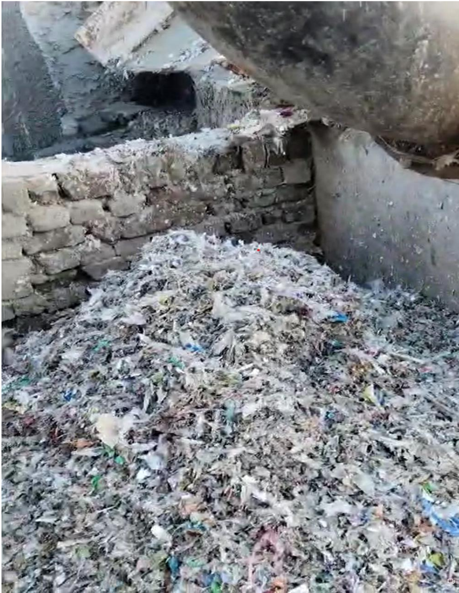
Collection of plastic from rotating drum
